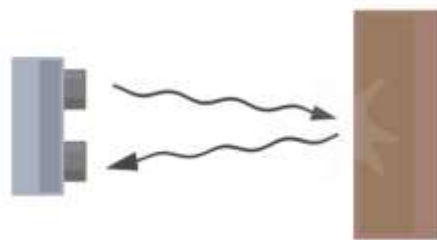
Figure (3-4) working principle of an ultrasonic
